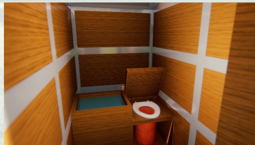
Modul B Composting Toilet
