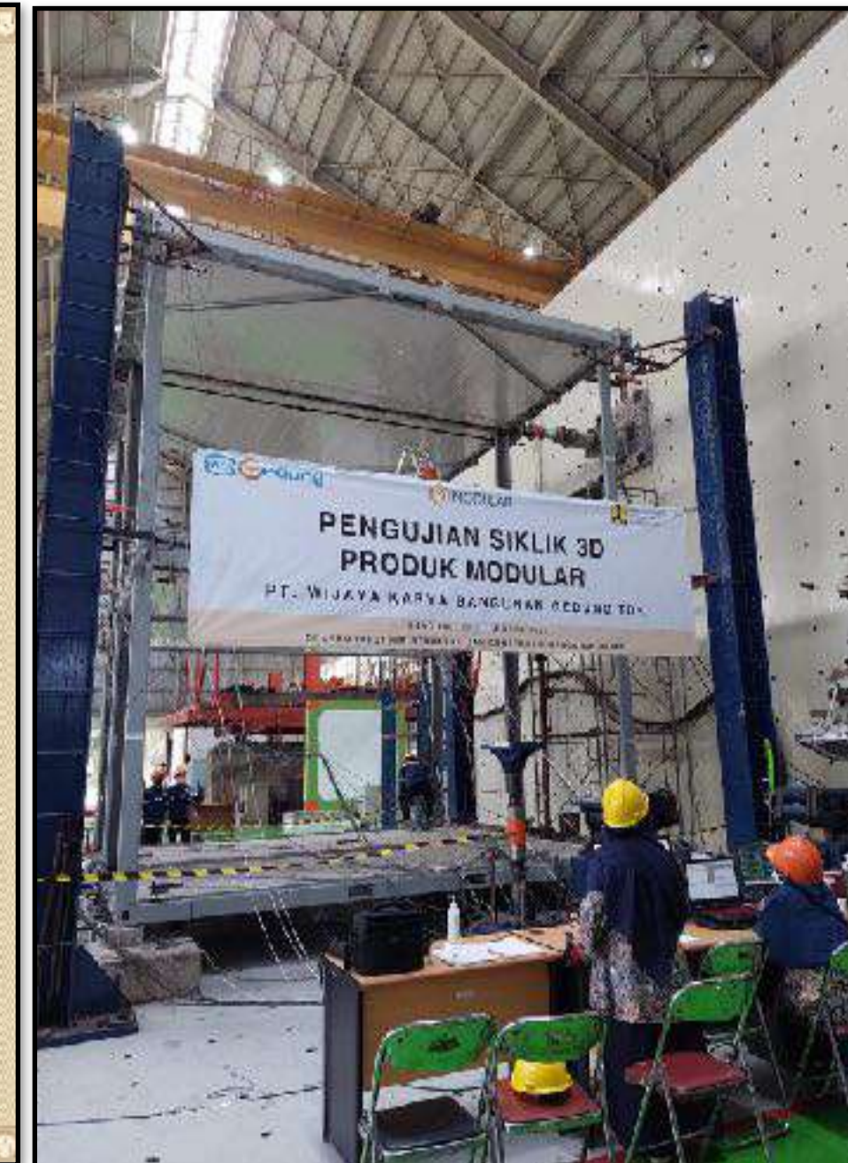
Has Passed Cyclic Testing from the PUPR Research Institute
